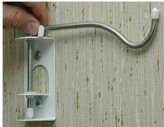
The bracket is made from 20 gauge steel and then it is powder-coated white. The rod is a stainless-steel 1/4" rod. The recommended maximum capacity for the assembly is 20 lbs. when the bracket is mounted securely to a stud or other solid structure. If you are mounting only into drywall with dry wall anchors, we recommend keeping the load less than 10-15 lbs because the quality of drywall/sheetrock can vary greatly.
